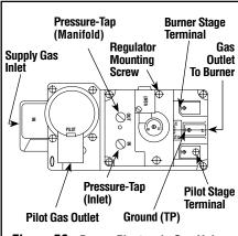
Figure 59 - Dexen Electronic Gas Valve
